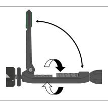
6. With cable clamp locked, start tensioning the system using the turnbuckle. Fold out handle to apply final tensioning force by rotating the turnbuckle as shown.
