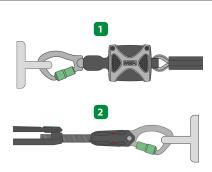
4. Connect energy absorber end of lifeline to anchorage point first [1], followed by the turnbuckle end [2].
